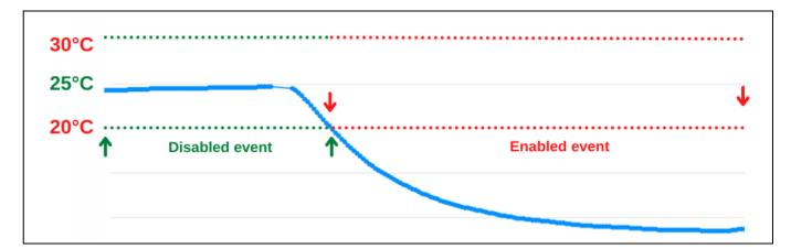
The frequency of messages sent when the temperature is out of the threshold (When the event is enabled) is configured by the user, so, if it is chosen a 5 minutes period, the device will send new event messages every 5 minutes.
